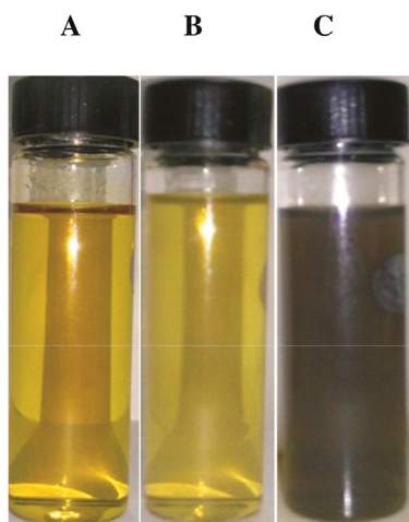
Fig. 6. Spectra and optical images of AgNCs in absence (■) and presence of starch (●) and effect of [electrolytes] = 0.04 \text{ mol dm}^{-3} on the position surface Plasmon resonance band. Reaction conditions: [\text{NaBH}_4]/[\text{Ag}^+] = 0.2 , [starch] = 1.0 \text{ cm}^3 of 2%.
